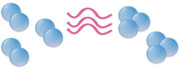
OXYGEN MOLECULE O<sub>2</sub> (Pure Oxygen) OZONE MOLECULE O<sub>3</sub> (Enriched Oxygen) THE THIRD ATOM ATTACHES TO THE POLLUTANT TO OXIDIZE IT TO A HARMLESS MOLECULE
